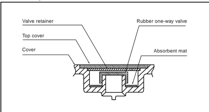
During ordinary use of the battery, the vent valve is closed to shut out outside air and prevent oxygen in the air from reacting with the active material in the negative electrodes.
